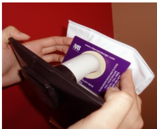
slide the collar of the dust bag over the black pipe
