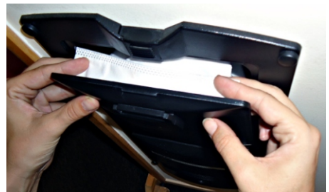
push the top edge of the bag inside the vacuum when closing the door
