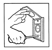
the best time to plumb in a central vacuum tubing system. Locate the inlet valve locations and nail the mounting plate to the nearest stud. Make sure the middle of the mounting plate is at the same height as the middle of adjacent electrical outlets.
