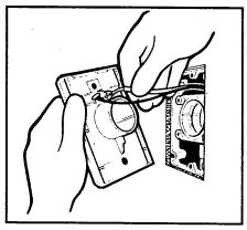
mounting plate by cutting off the plastic rivets with side cutters. Tape low voltage wire to the end of a sufficiently long piece of tubing and pass it up from beneath. If the trunk line is in the attic, tie a weight to the end of the low voltage wire and lower it through the opening. Remove the wire and pass it through the upper hole in the
