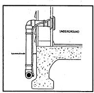
assemble and test the tubing and low voltage wire before filling in the trench. It is recommended that the low voltage wire installed outside be encased in conduit which is available at most hardware stores.
