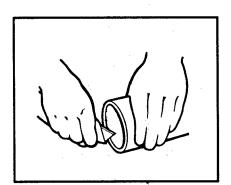
**Gluing:** PVC solvent cement actually welds the fitting to the tubing. A chemical reaction permanently joins the molecules from each surface to produce an airtight seal.
