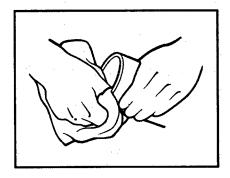
This bead will reduce airflow and could cause a clog. The tubing should be inserted all the way into the fitting and twisted a quarter turn to evenly distribute the cement. All excess cement should be removed with a rag. The glue should be allowed several hours to set before the vacuum system is used.
