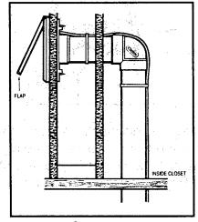
assembly to the wall as described above. From inside the closet insert short piece of tubing into the coupling. Dry fit a tight 90 degree fitting pointed in the direction of the trunk line. Cut 1/2" hole 2 directly below the
