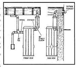
\*\*Vacuums must breathe ... do not enclose. If the unit is to be located in a closet or utility room it must be vented. Louvered doors fulfill this purpose. A muffler can, of course, be used to minimize noise.
